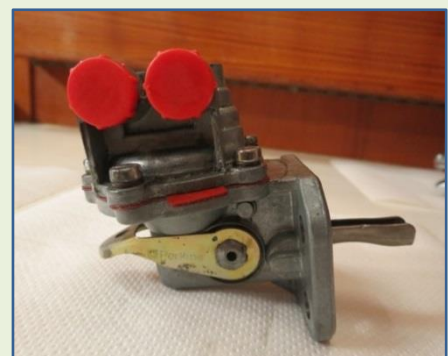
The old lifting pump removed
