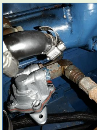
Fuel lifting pump in situ
