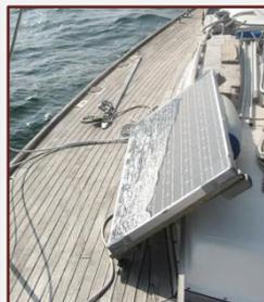
under sail, the towing generator gave us many amps. Once, due to lack of space, the solar panel was transported from the storage inside Zeezwaluw to the top of the turned dinghy. Riens fitted a 12V socket in an extension of the air-vent and a second regulator. Now the solar panel was also able to help the towing generator to charge the batteries. This combination produced so much energy that the
