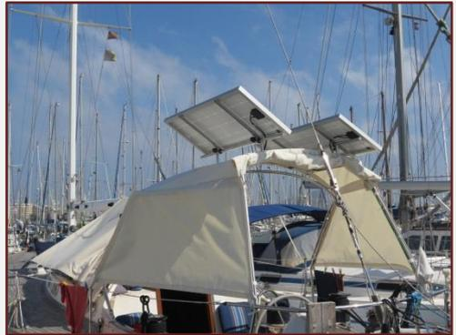
Due to the fact that we are still in the marina and connected to 220V shore power, there was no need for working solar panels. To stop them working, we made 2 covers out of the same Sunbrella as the bimini. After the covers were produced and put on the panels, they were still producing amps!!!! Yes the sun went straight through the beige fabric, who would have thought about that!
