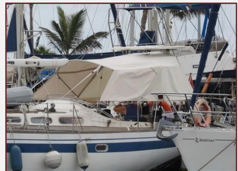
tightened down with webbing and clips where necessary. The last and final project was to sew shade-cloth (kind of netting) into the back and 2 aft panels. The 30cm of this cloth gave us more visibility while it kept 90% of the sun out but let the wind through. The end result turned out to be perfect.
